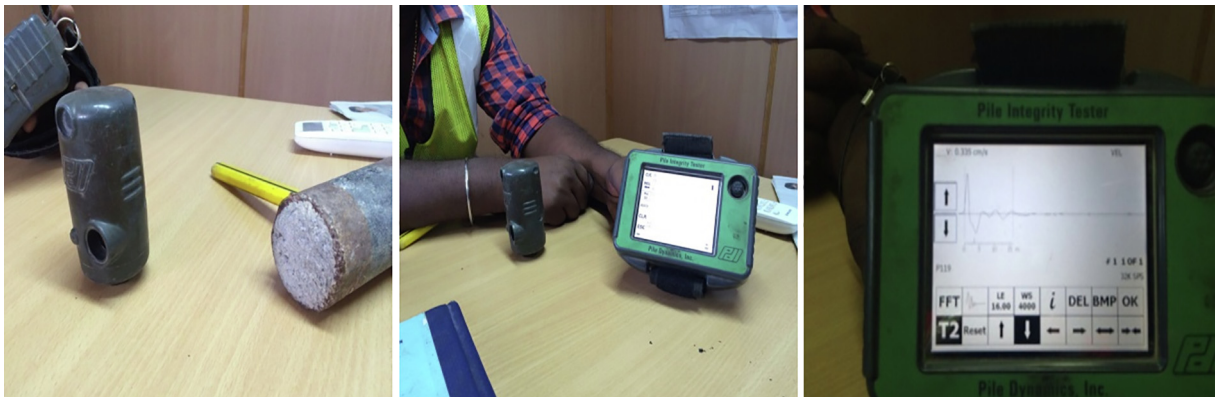
Fig. 2. Pile integrity test.
